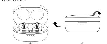
When using the FW3 for the first time, open the charging case, the white lights of the two units will be continuously on for about 3s, and then the FW3 will turn on automatically and enter Bluetooth pairing mode. At this time, your device can search for and connect to the "FiiO FW3". In follow-up uses, it can automatically reconnect to this device once being powered on. ②Charging when powered off: Put the two units into the charging case and close it. The FW3 will automatically
